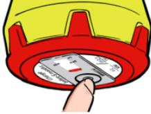
7. Mark the b.safe Waste Cap with a foil pen or an adhesive label if necessary.
