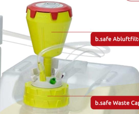
A photograph of a laboratory waste filter assembly. It consists of a yellow plastic cap with a red top, mounted on a white plastic base. A clear plastic tube is connected to the side of the cap. The assembly is mounted on a white plastic container. The background is white with a yellow curved shape at the bottom right.
