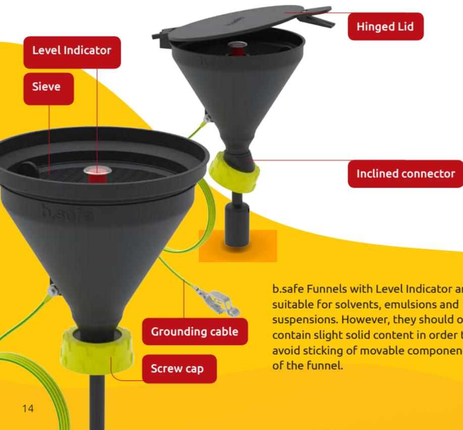
b.safe Funnels with Level Indicator are suitable for solvents, emulsions and suspensions. However, they should only contain slight solid content in order to avoid sticking of movable components of the funnel.
